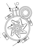
Remove screws securing the electric cover to the back sheet and remove cover and disconnect the terminals from the rear.
